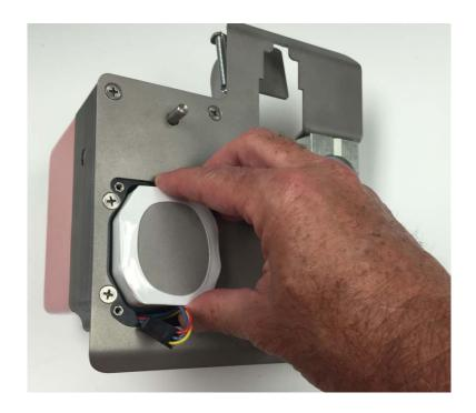
**STEP 5** – The battery connector should be in the space provided as shown below
