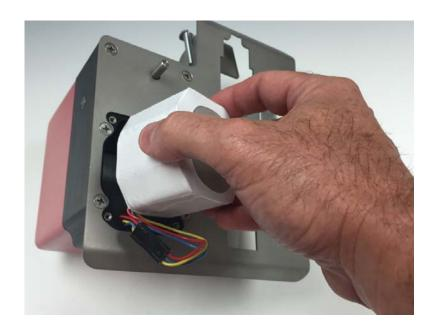
**STEP 3** – Disconnect battery at connector.
