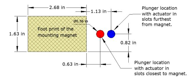
With the plunger in the retracted position, the actuator can be infinitely adjusted so that the plunger is anywhere from 0.30" to as much as 1.40" above the magnet mounting surface (which is normally the surface of your equipment). The plunger can extend up to 2".
