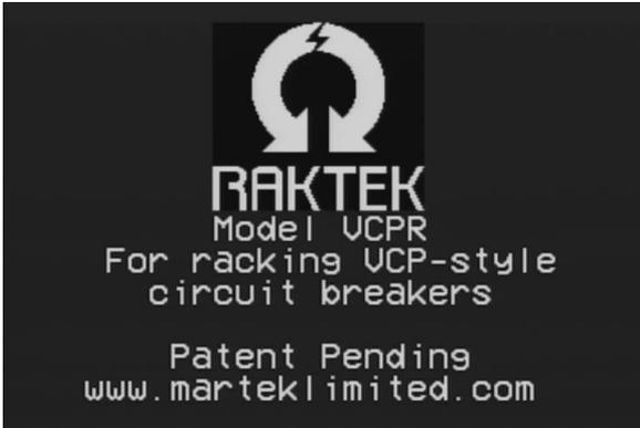
*Upon powering-up the VCPR, the introductory screen will appear. Pressing the Enable button for one second will advance the display to the next screen.*
