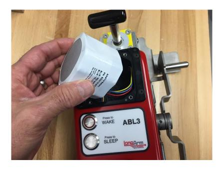
**STEP 3** – Disconnect battery at connector.
