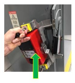
Use a similar (reverse) action when the disconnect handle is in the UP position. Start at the top, slipping the actuator arm behind the disconnect handle. Rotate the ABL3 downward.
