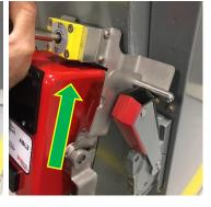
**STEP 4** -- Disconnect cable (for cabled versions only) and return components to carrying case or store on the side of the MCC. (See Section 5.0 for details)
