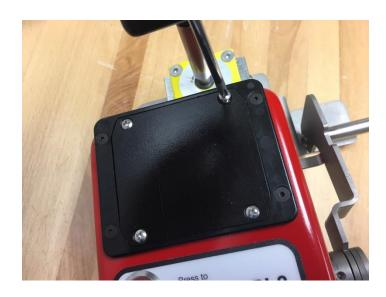
**STEP 2** – Remove battery cover plate and slide battery out.
